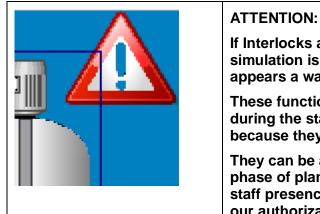
If Interlocks are OFF or the software simulation is ON on the top right of the page appears a warning icon
