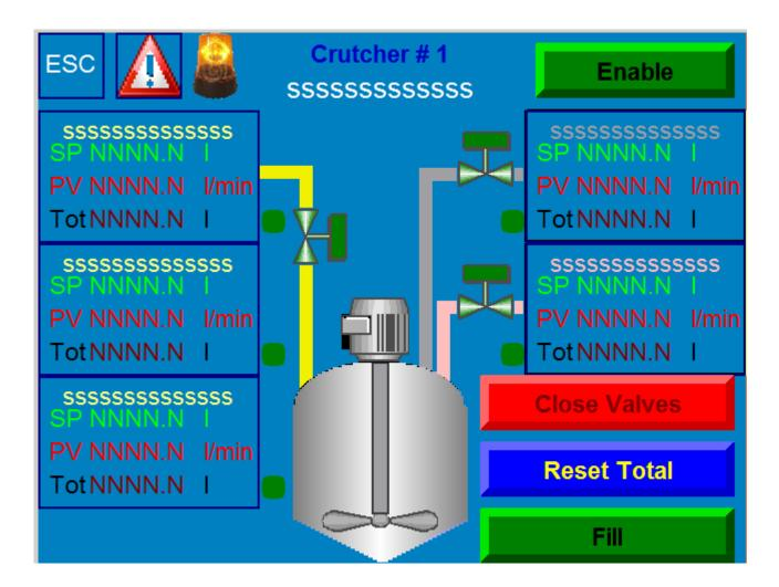
On the Bottom right the "Close Valves" command close the three inlet valves
